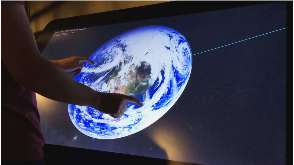
Figure 1.1: 3D Astronomical Visualization software OpenSpace using multi-touch to control the view in six degrees of freedom (DOF).
